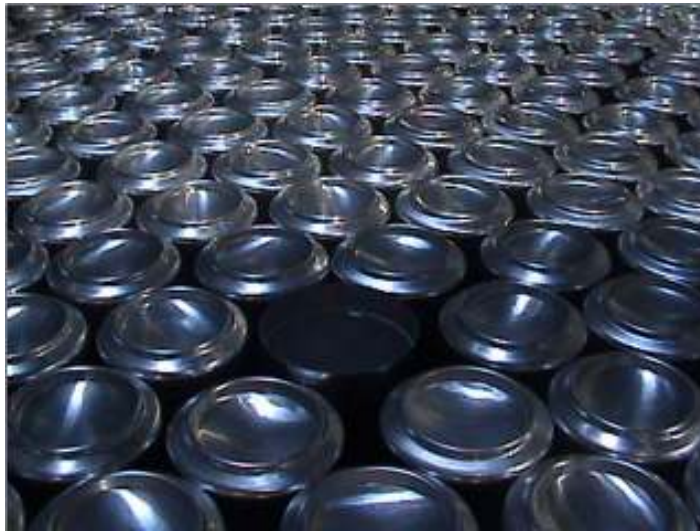
Figure 2. The upturned can contaminating the other neighboring cans
